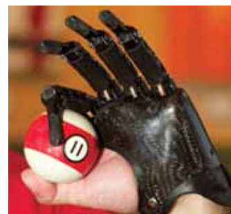
Innovative prosthetic technology Individually articulating electronic fingers are a break-through in prosthetic technology.
