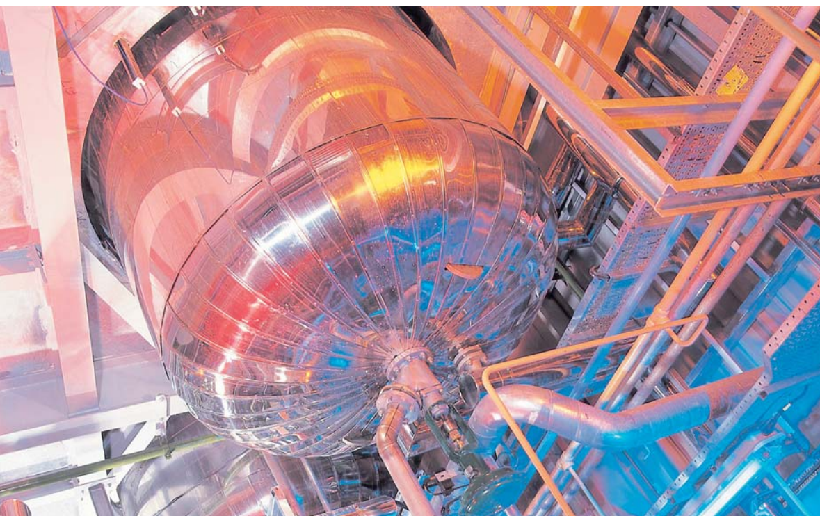
▲ Smooth reaction: Chemical reactors at the Workington site of Pentagon Chemicals, manufacturing a batch of methyl magnesium chloride. The product is used in the synthesis of a flavouring for cough mixture. Each vat is four cubic metres.
