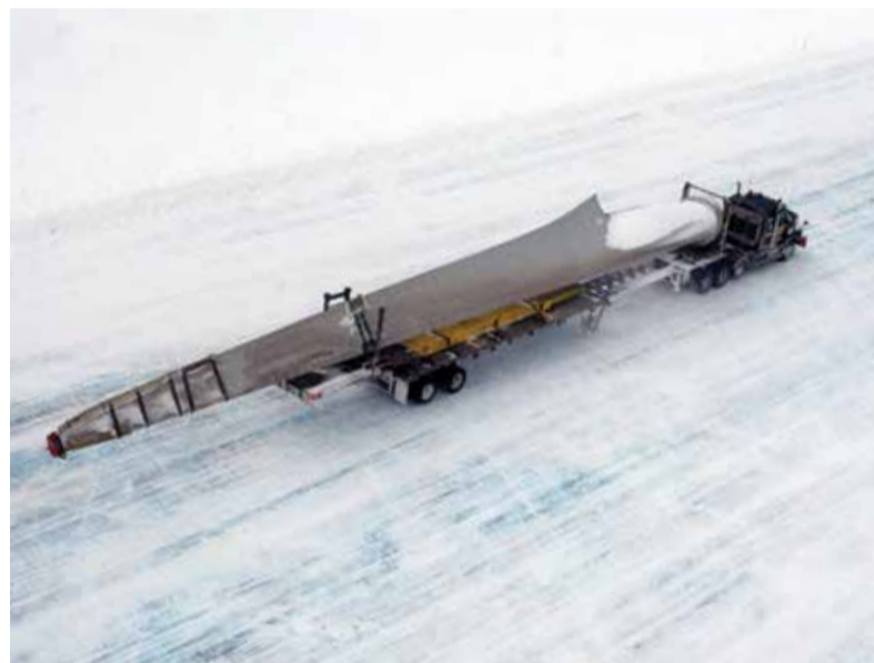
► EFFICIENT AND CLEAN TOP: Farming fields provide a perfect venue for wind turbines. BOTTOM: A truck transporting a wind turbine blade over an ice road in a remote community. PHOTOS: CANWEA
